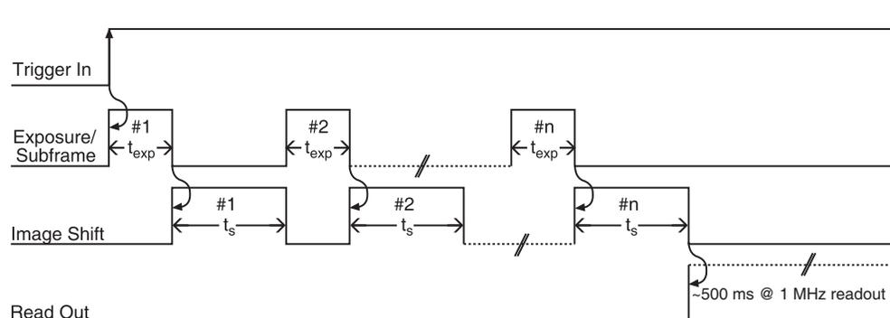
In multiple trigger {Shift Per Trigger} mode, each exposure-shift cycle is triggered independently by a pulse applied at the **Ext Sync** connector. This mode is useful when each subframe needs to be synchronized with a pulsed external light source such as a laser. [Figure 6-14](#) illustrates the timing diagram.
