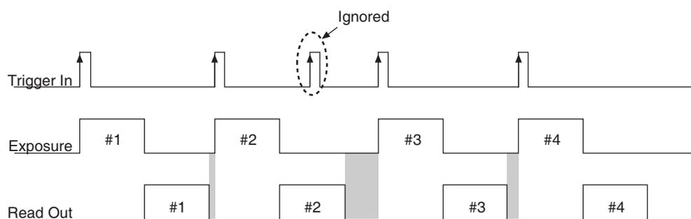
For a sequence of one frame, bulb mode and trigger-first mode are the same. The shaded areas
