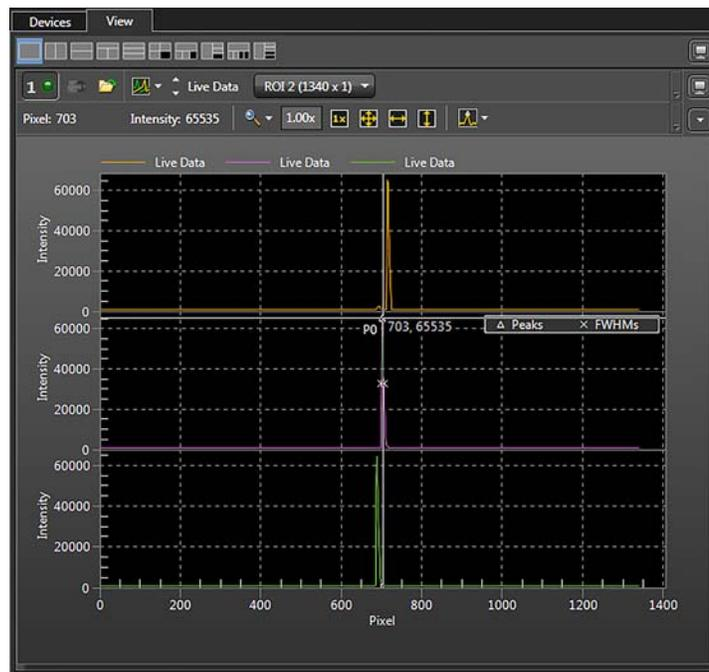
7. Slowly move the camera in and out of focus. You should see the spectral line go from broad to narrow and back to broad. Leave the camera set for the narrowest achievable line. Note that the Peak Finding function is active for the center graph to allow you to monitor the FWHM information to achieve the narrowest line width. The way focusing is accomplished depends on the spectrograph, as follows:
