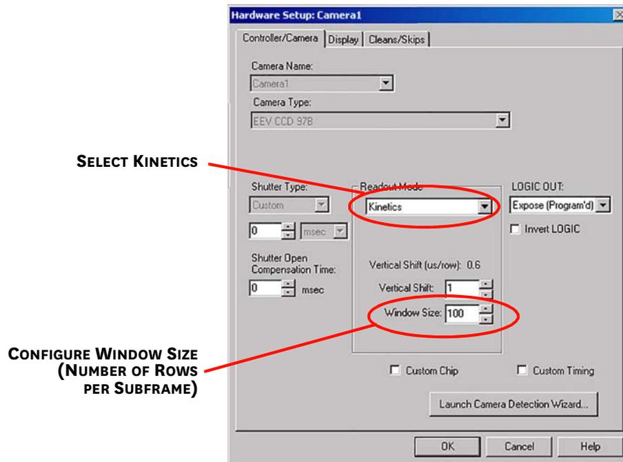
Figure 6-11: Typical LightField Sensor Expander: Kinetics Readout Mode
