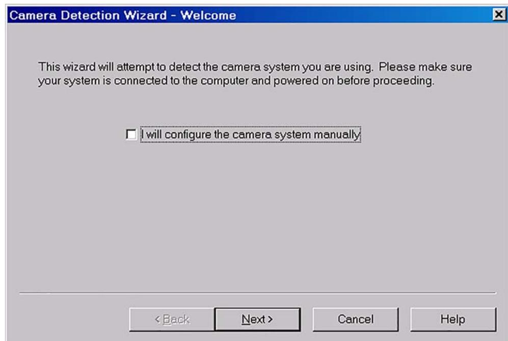
4. Follow the instructions on the dialogs to perform the initial hardware setup: this wizard enters default parameters on the Hardware Setup dialog tabs and gives you an opportunity to acquire a single test image to confirm the system is working. Note that this is a test image and it is not acquired using the settings needed for true data acquisition.
