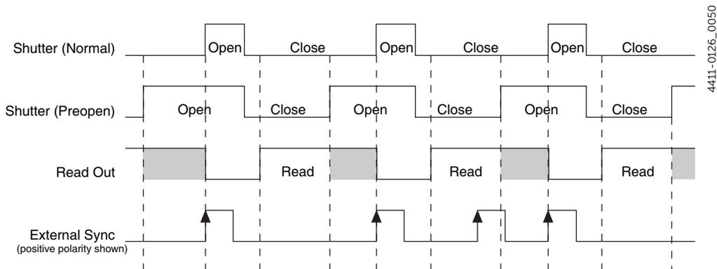
Figure 6-6: Timing Diagram: LightField Clean Until Trigger (CUT)
